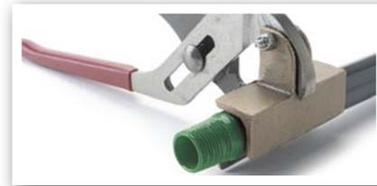
**Z-Wrench** features extra wide jaws which spread the clamping force, enabling the tool to grip without marring the surface of the conduit. The "V" shaped upper jaw allows **Z-Wrench** to accommodate a wide range of conduit sizes. Shallow grooves in the upper and lower jaws provide an excellent grip.
